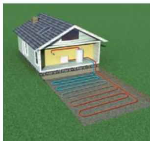
GSHP Ground source
